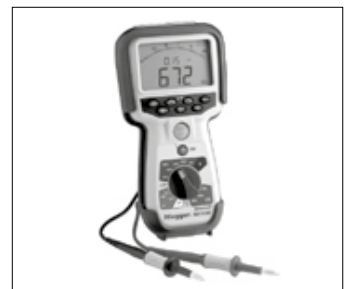
Megger control appliance for alarm wires. See Chapter 8.
